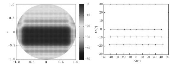
Beam spatial arrangement in the sinusoidal space coordinate system without radar inclination
