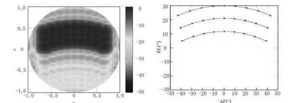
Beam spatial arrangement in the sinusoidal space coordinate system with  $30^\circ$  radar inclination
