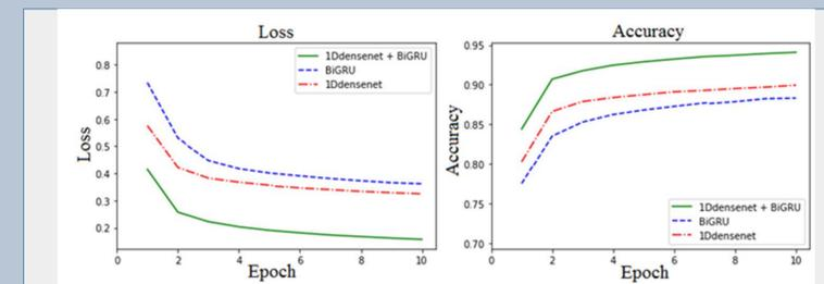
Fig.2 Comparison of loss values and accuracy curves of three models
